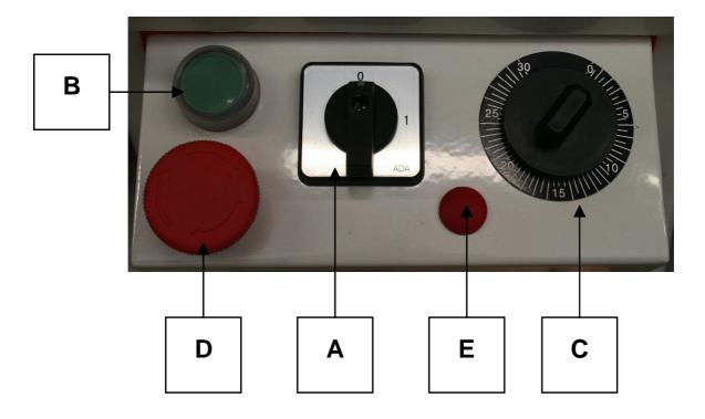
The panel consists of a main switch (**A**), a green start button (**B**), a timer (**C**), a red emergency stop button (**D**) and a speed adjustment knob (**E**).
